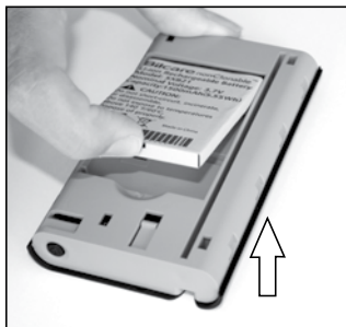
Fig. 3: Should you need to remove the battery at some stage, push slightly back towards the connector and up.
