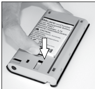
Fig. 2: Insert the battery by pushing slightly towards the connector and down.
