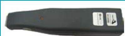
Figure 3. A handheld Singular ID scanner which connects to a standard mobile phone to access the remote database.
