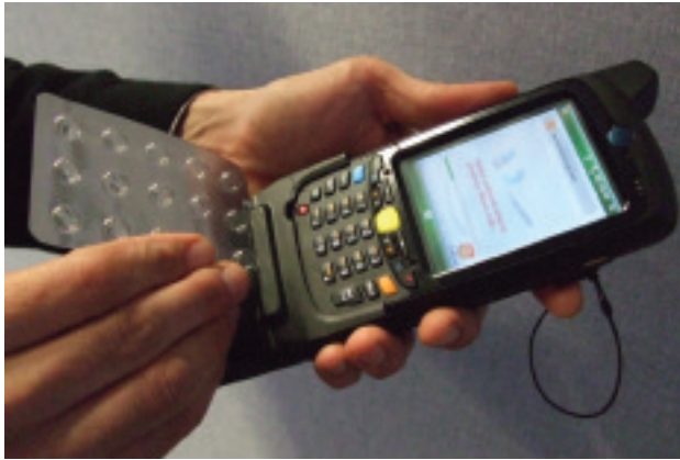
Figure 4: A handheld industrial PDA with integrated clip-on device for authenticating, amongst other things, pharmaceutical blister packs
