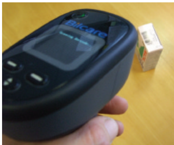
Figure 1: A device capable of reading barcodes (above) as well as authenticating a security feature on a packet (right)
